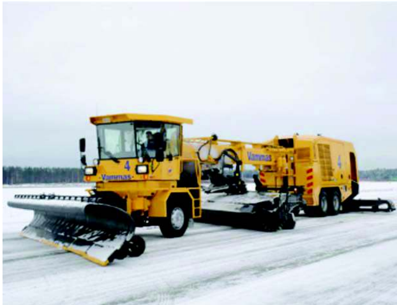
Figure 16E-9 Two-Way Snowplow Blade Mounted on a Special Chassis
