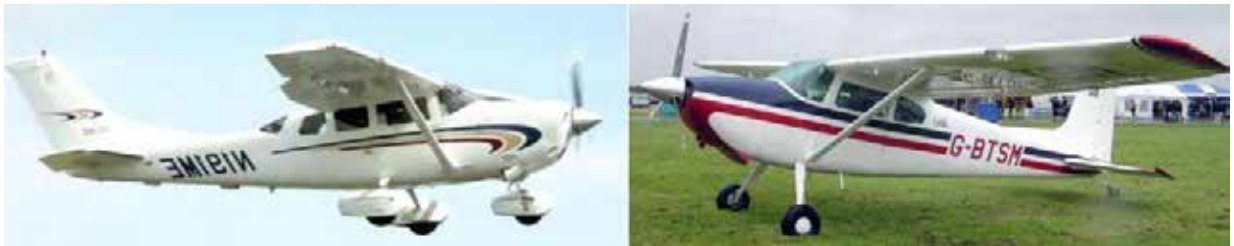
Figure 3 Nose Gear v. Tail Gear
