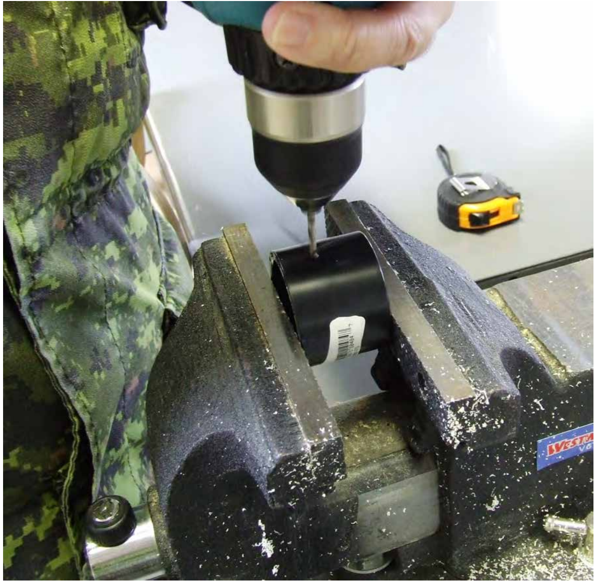
Figure 26-A Drilling 1/8-inch Holes in the ABS Coupler
