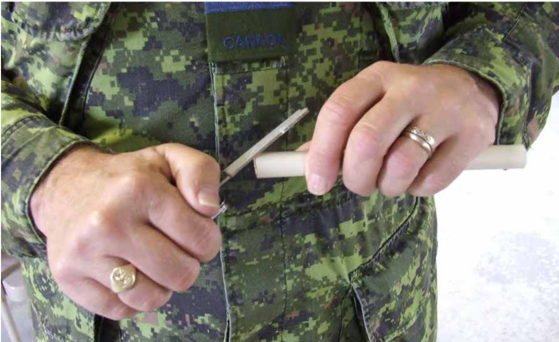
Figure 5-A Deburring the end of the tube with a hand file.
