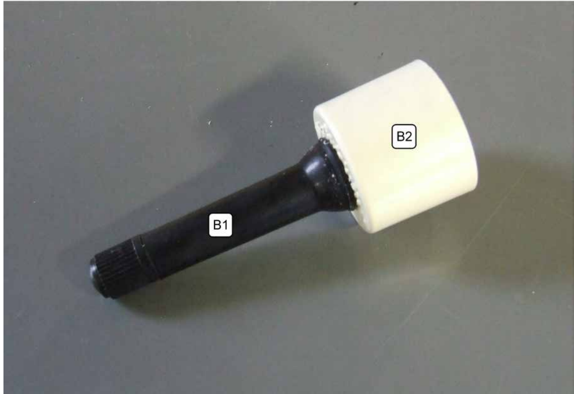
Figure 12-A Section B, Tire Valve Pulled Through B2
