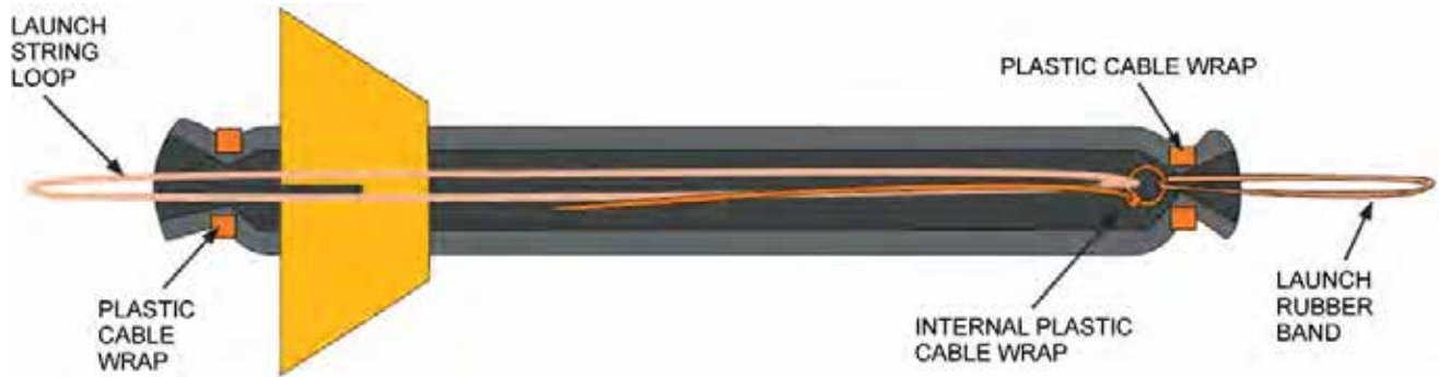
Figure 1 Exploded View of the Foam Rocket
