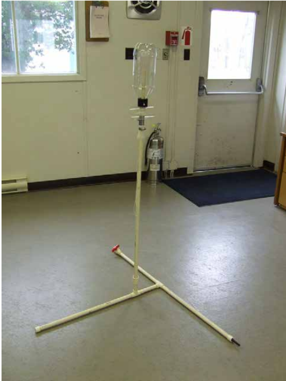
Figure 33-A Assembled Water Rocket Launch System
