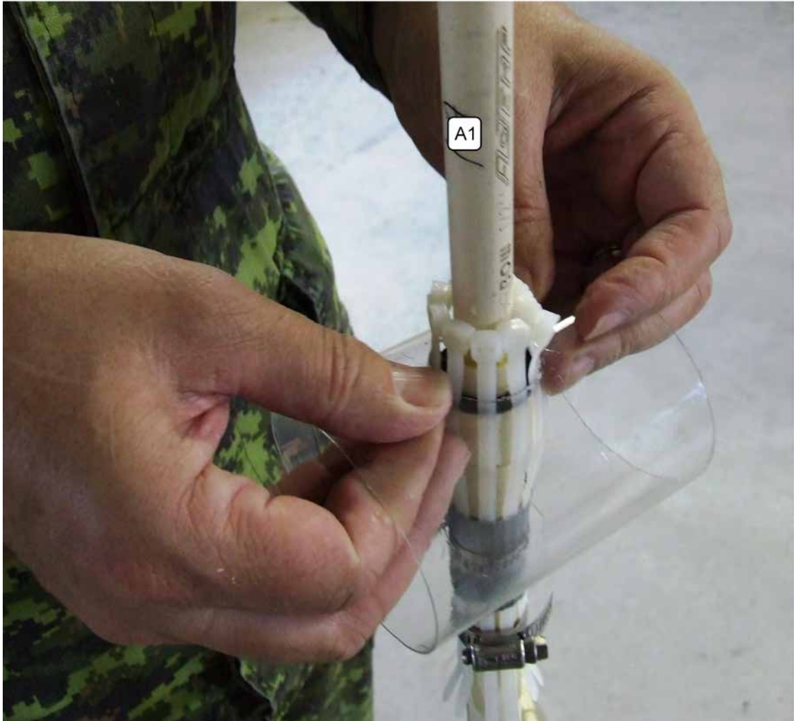
Figure 28-A Sliding the Spring over the Cable Ties
