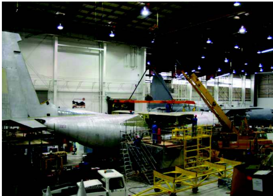
Figure A-2 Placing a C-130 Centre Wing
