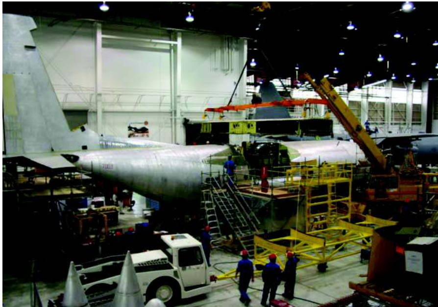
Figure A-1 Rebuilding a C-130 Centre Wing
