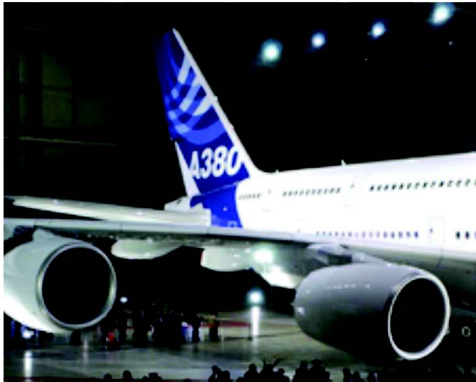
Figure B-5 Engines on Pylons
