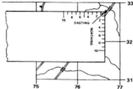
Figure 18 Using a Constructed Romer
