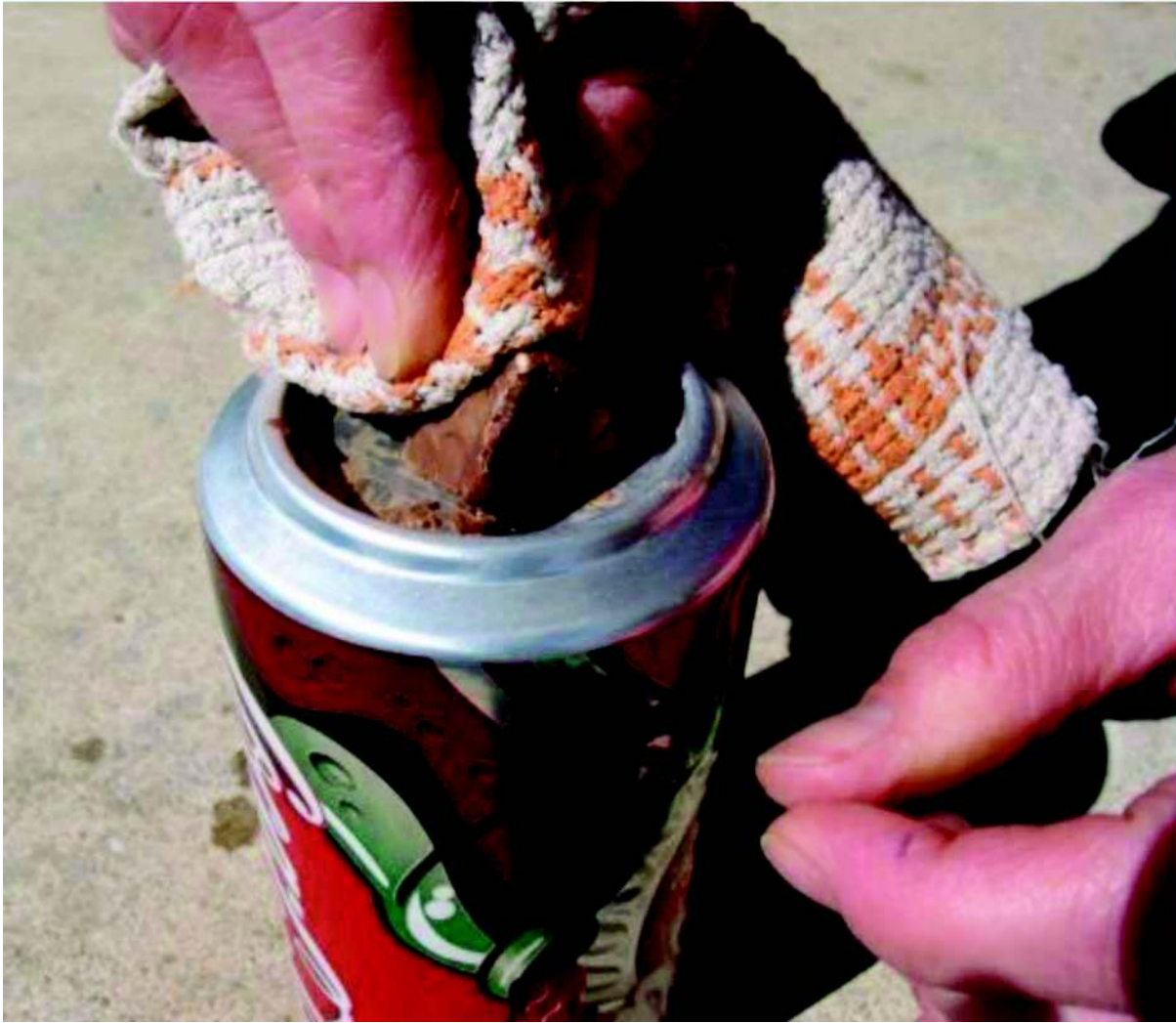
Figure 4 Polishing the Aluminum Can Bottom
